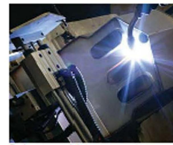
Robotic welding is precise, virtually eliminating leaks.
